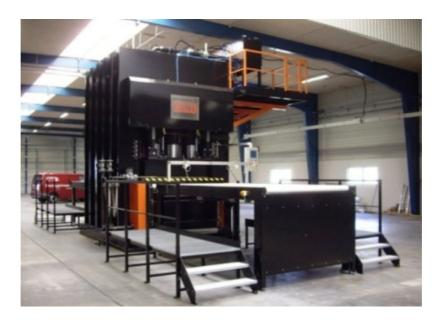
Very solid all-welded frame construction for carrying press platens, upper as well as lower. Each frame is prepared in one setup that secures a parallel installation of the press platens.
