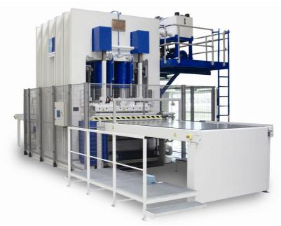
Very solid all-welded frame construction for carrying press platens, upper as well as lower. Each frame is prepared in one setup that secures a parallel installation of the press platens.
