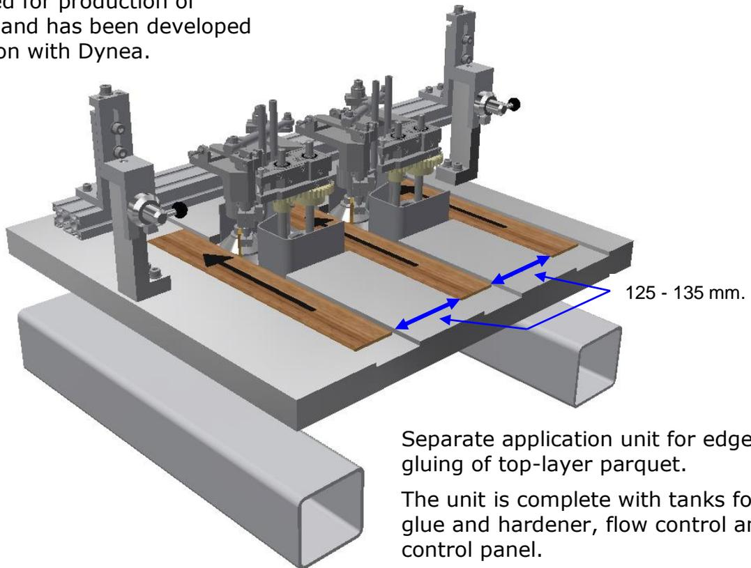
Separate application unit for edge gluing of top-layer parquet.
